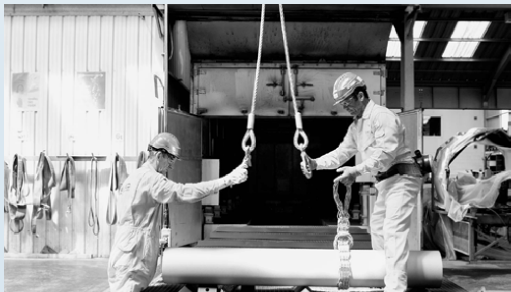
Heated pipe before application of epoxy powder
