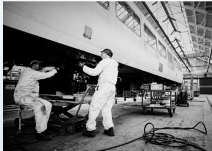
Replacing the air conditioning technology on a train of the type 156.
