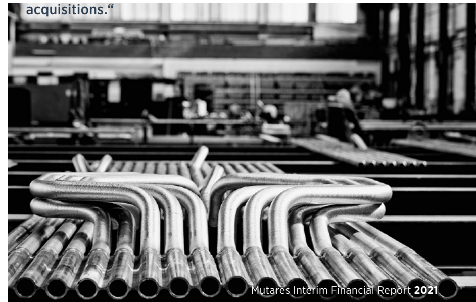
Pipe bends as part of a replacement of boiler pressure parts
