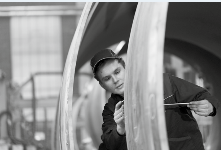
Balcke-Duerr: measuring coat shots for high pressure preheater
