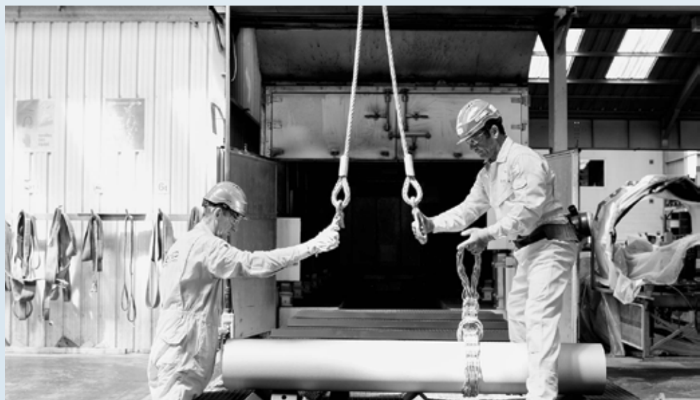
Heated pipe before application of epoxy powder
