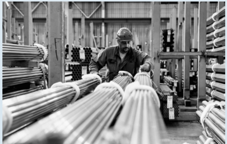
Bundling and final inspection of the stainless steel pipes before shipment
