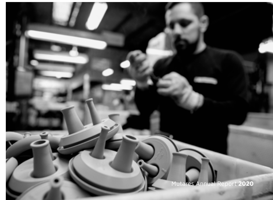
Final quality inspection of a dash grommet
