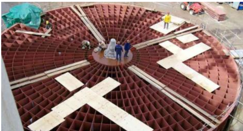
21m-diameter air preheater for Walsum, Germany
