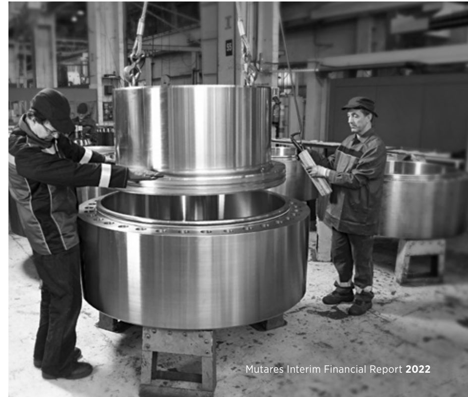
Adjustment of piston in a roll force cylinder for Rolling Mill in Clecim's workshop
